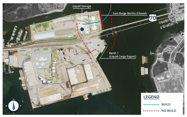
Figure 2. With the East Barge Berths closed, liquid barges must navigate to Berth 1 beneath the Newport River Bridge, which requires a skilled pilot and fair weather. Liquid cargo must travel a longer distance to be unloaded, use inefficient temporary equipment at Berth 1, and there is no capacity to stage more than one barge for unloading at a time nor load an export ship while barges are unloading.
