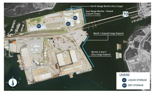
Figure 1. The project scope includes reconstruction of the Phosphoric Acid Terminal North and East Barge Berths to restore state of good repair, safe working conditions, and full berthing capacity.
